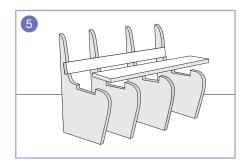
**5.** Take the Seat Support piece (**Part D**) and firmly press it into these recesses.
