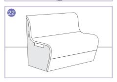
20. Apply adhesive to the remaining areas of the Support Profiles and press the Front Board into place.
